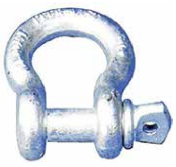
PEERLESS SHACKLES • Hot dipped galvanized to ASTM A153 • Proof load at 2 times the working load limit • Ultimate load at 5 times the working load limit • Meet or exceed FED SPEC RR-C-271D requirements • 5/16", 3/8", 7/16", 1/2", 5/8", 3/4", 7/8", 1", 1-1/8", 1-1/4", 1-3/8", 1-1/2", & 2"
